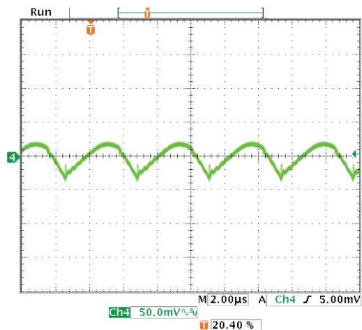
Step Load Transient Response (Vin=48V, Vout=nom., Iout=50-75-50% of full load, Cload=1 uF ceramic II 10uF tantalum, Ta=+25°C., ScopeBW=20MHz Ch1=5Vo, Ch2=Io 2amps/div)
